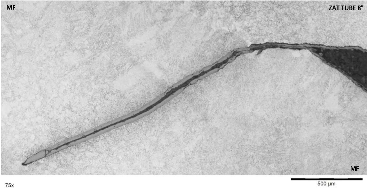
FIGURE 59 DETAIL 1 DE LA FIGURE 58 FISSURATION EN ZONE FONDUE
