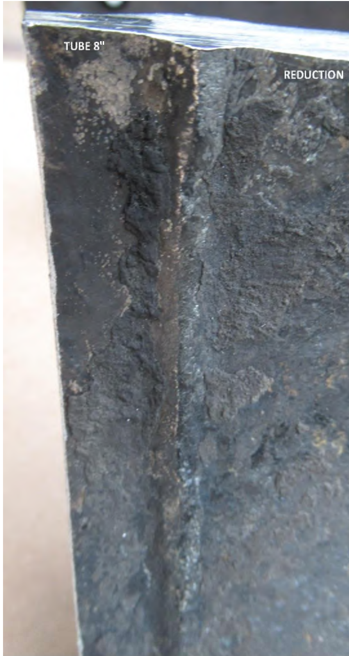
FIGURE 17 DETAIL 5 DE LA FIGURE 10 SOUDURE TUBE / REDUCTION
