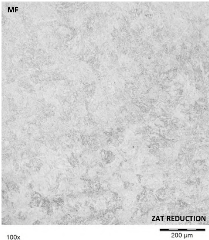
FIGURE 55 DETAIL 5 DE LA FIGURE 46 ZONE DE LIAISON COTE REDUCTION
