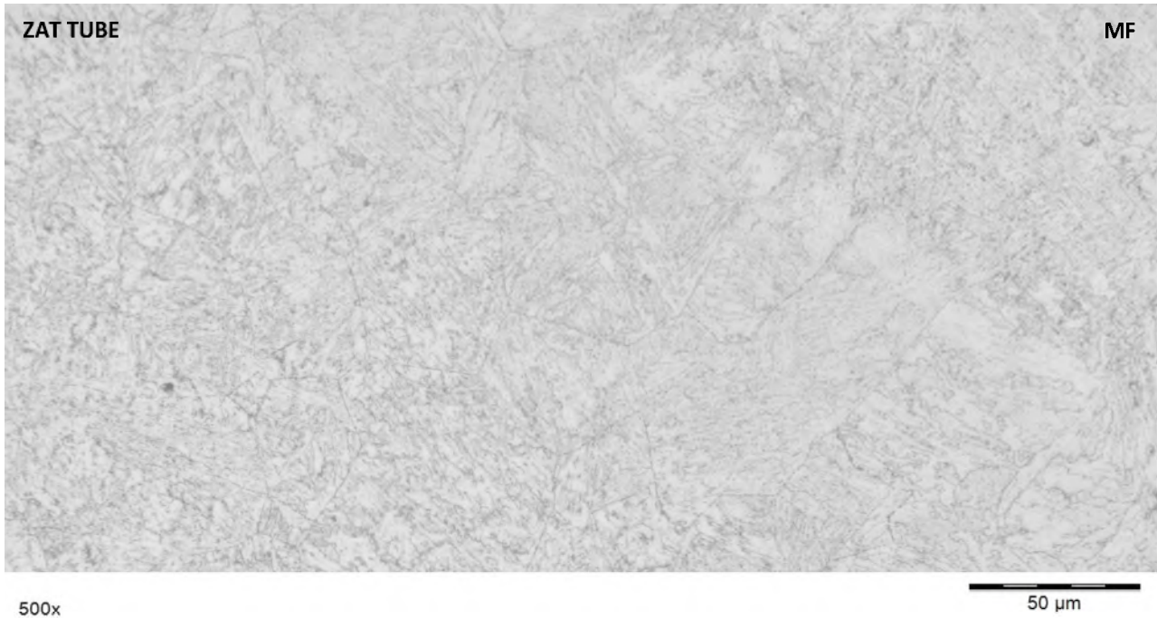
FIGURE 54 DETAIL 4 DE LA FIGURE 46 ZONE AFFECTEE THERMIQUEMENT COTE TUBE
