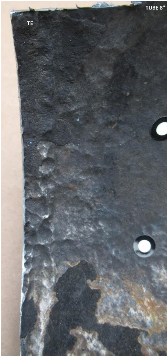
FIGURE 11 DETAIL 1 DE LA FIGURE 10 SOUDURE TUBE / TE
