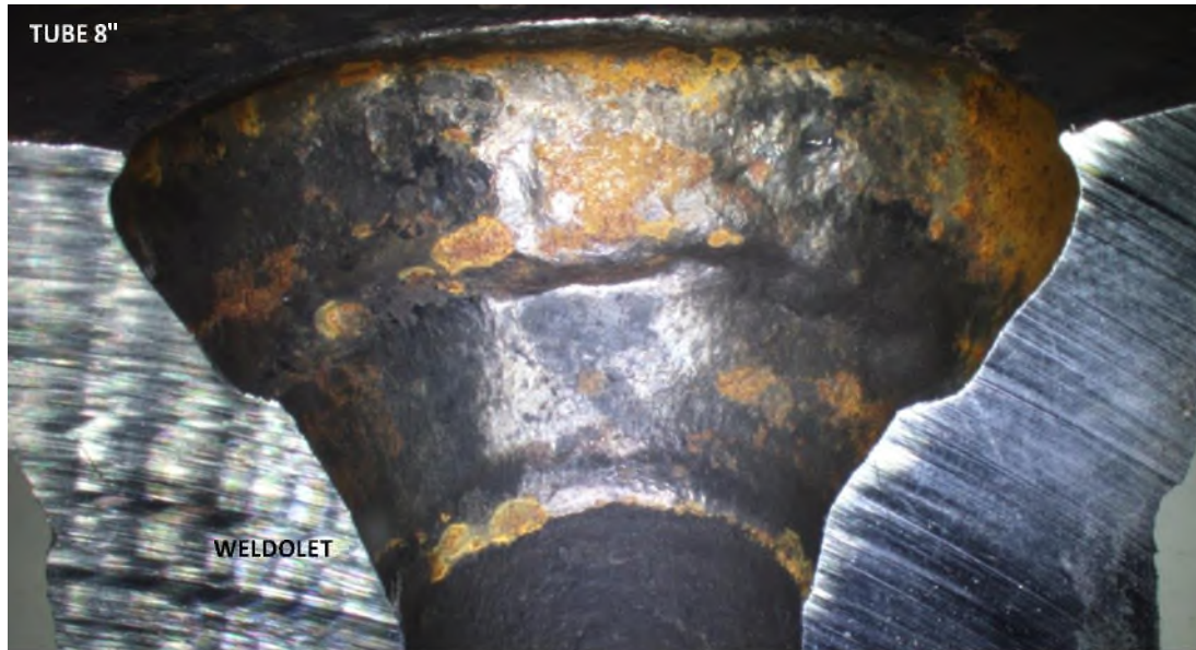
FIGURE 6 DETAIL DE LA FIGURE 5 SURFACE INTERNE DU PIQUAGE 3/4" TUBE 8"
