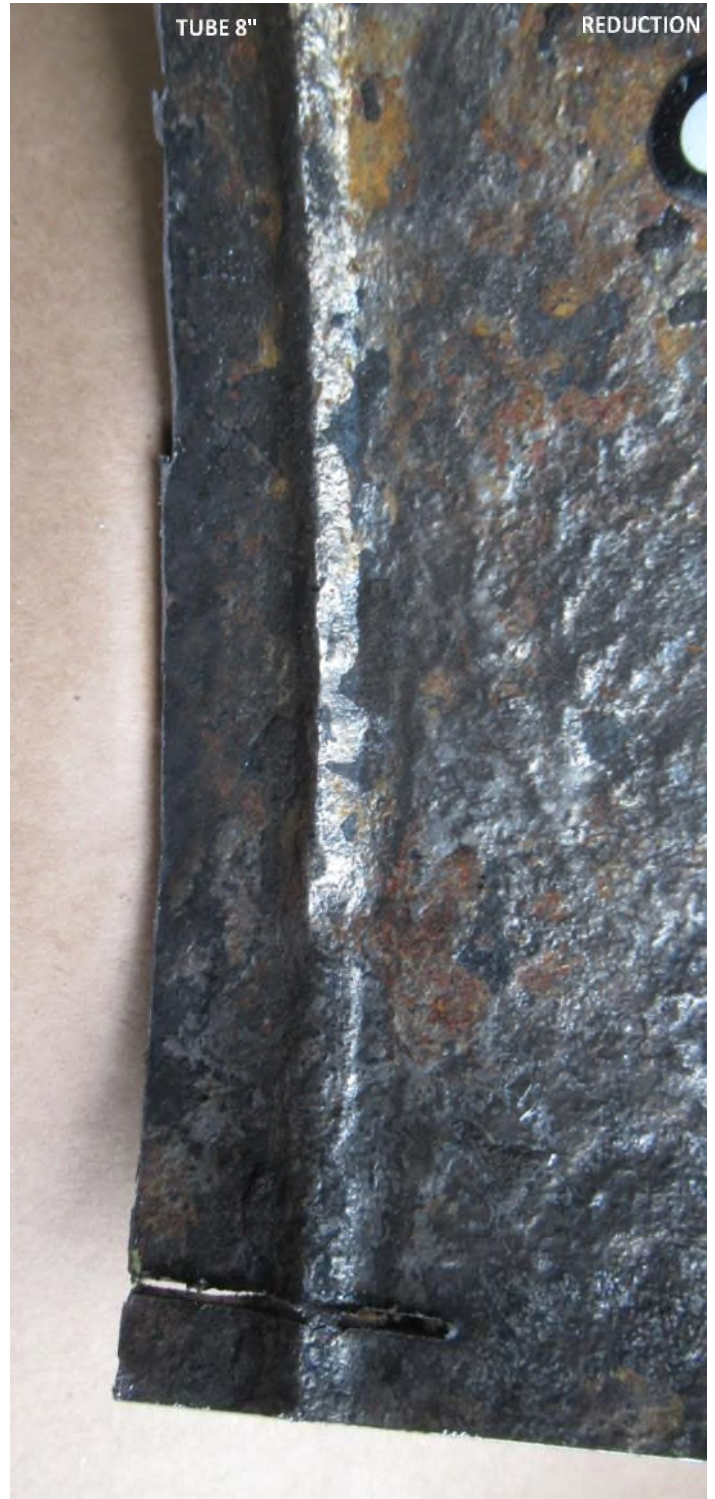
FIGURE 16 DETAIL 4 DE LA FIGURE 10 SOUDURE TUBE / REDUCTION
