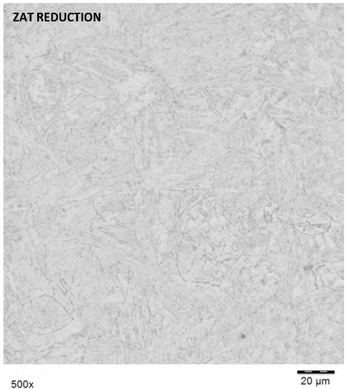
FIGURE 56 DETAIL DE LA FIGURE 55 ZONE AFFECTEE THERMIQUEMENT COTE REDUCTION
