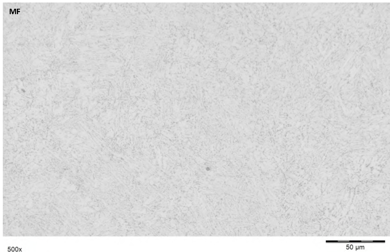
FIGURE 45 DETAIL 6 DE LA FIGURE 37 ZONE FONDUE COTE INTERNE
