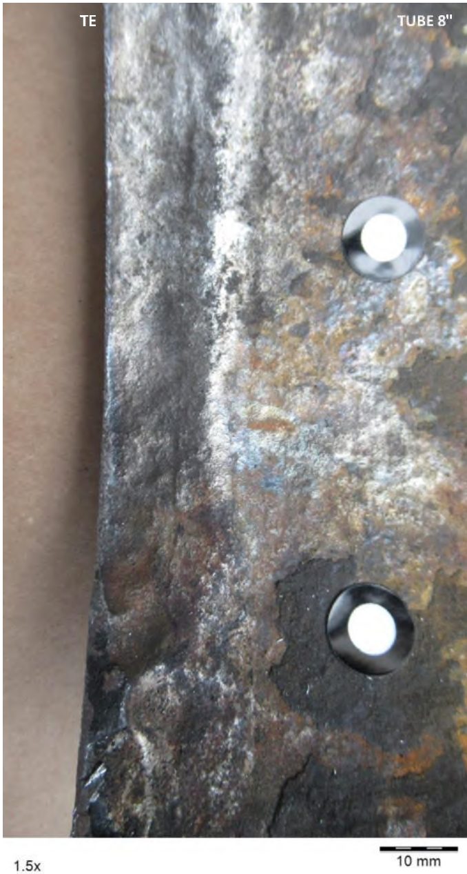
FIGURE 13 DETAIL 2 DE LA FIGURE 10 SOUDURE TUBE / TE
