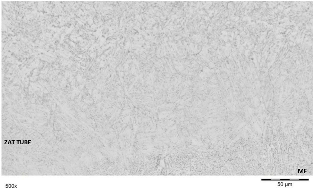
FIGURE 64 DETAIL 2 DE LA FIGURE 58 ZONE AFFECTEE THERMIQUEMENT COTE TUBE
