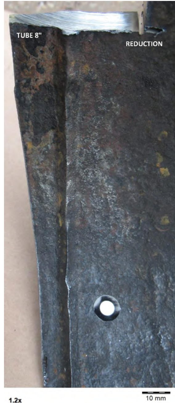
FIGURE 14 DETAIL 3 DE LA FIGURE 10 SOUDURE TUBE / REDUCTION
