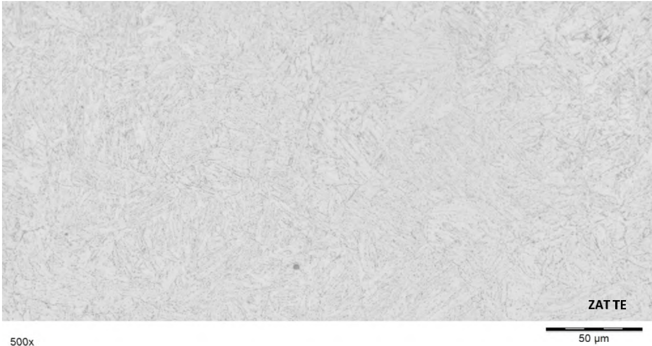
FIGURE 42 DETAIL 3 DE LA FIGURE 37 ZONE AFFECTEE THERMIQUEMENT COTE TE
