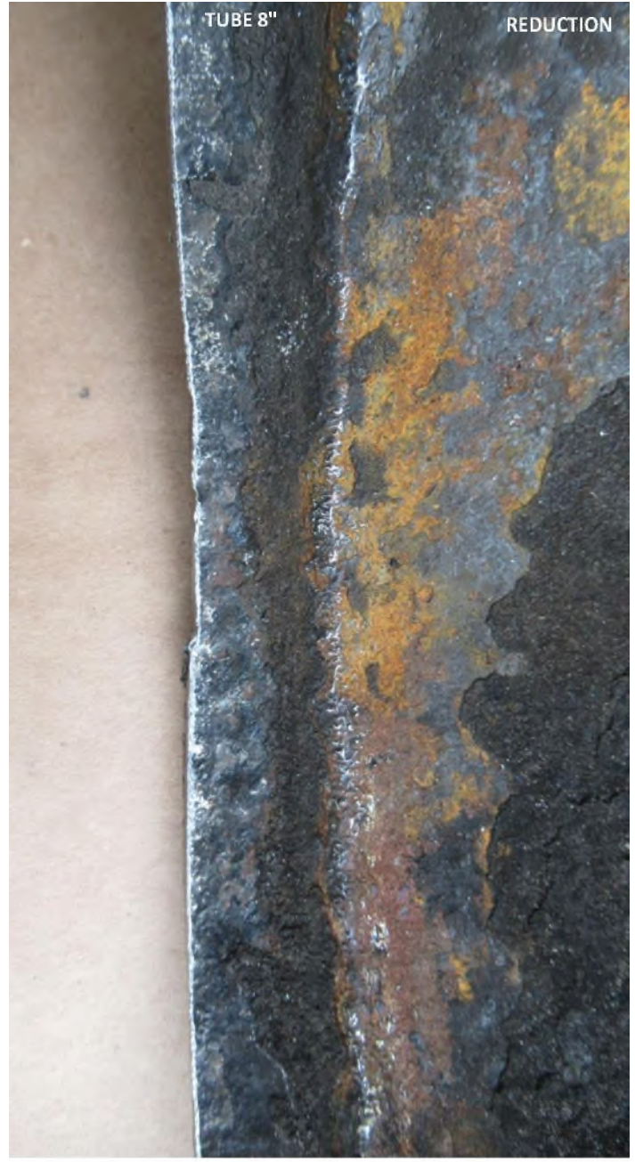
FIGURE 18 DETAIL 6 DE LA FIGURE 10 SOUDURE TUBE / REDUCTION
