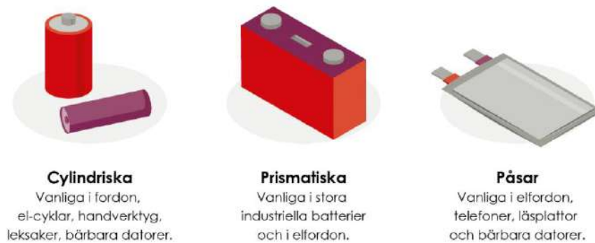
Figure 2. Appearance and presence of lithium-ion batteries.
